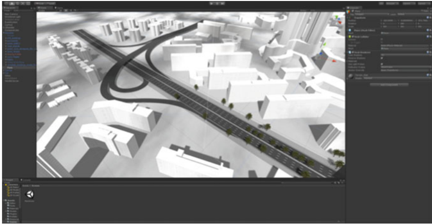
Fig. 5 Unity3D editor: The creator of the tool is able to import 3D models and change various parameters of the component ( right panel ). The components in the scene are listed on the left panel . The bottom panel shows the list of files that make up the project (textures, scripts, 3D model, images, audio, etc.)
