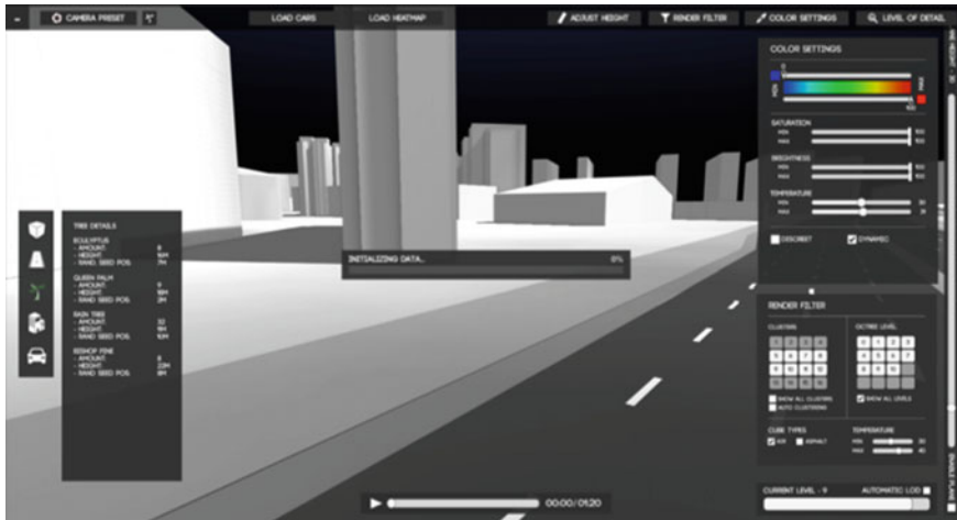
Fig. 3 Camera presets and views are necessary elements in every exploration tool. The info panel helps users to know the context of data and model. Filter and color settings help further to understand the information shown better
