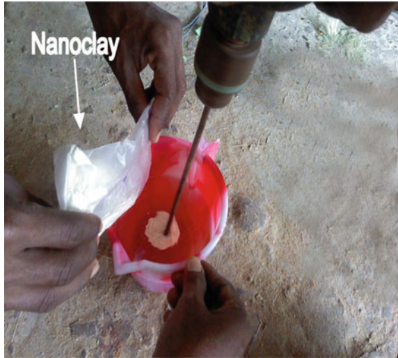
Fig. 3 Mixing of nanoclay with polyester resin
