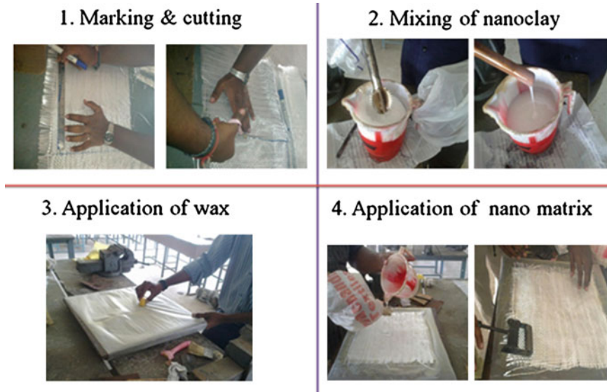
Fig. 5 Preparation of nano composites by hand lay-up process
