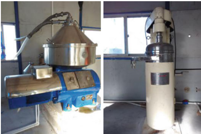
Fig. 5 Disk centrifuge (left), Tube centrifuge (right). Photos are taken from microalgae culture facilities of Guangzhou Institute of Energy Conversion, Chinese Academy of Sciences, China
