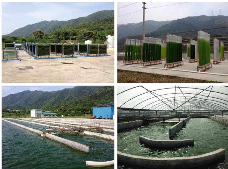
Fig. 1 Microalgae culture facilities of Guangzhou Institute of Energy Conversion, Chinese Academy of Sciences (GIEC-CAS), China. Flat plate photobioreactors (up-left), column photobioreactors (up-right), open pond culture (down)
