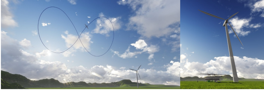
Fig. 26.1 Comparison of Ampyx Power's 2 MW AWES with typical 2 MW wind turbine in flight (left) and in storage (right)
