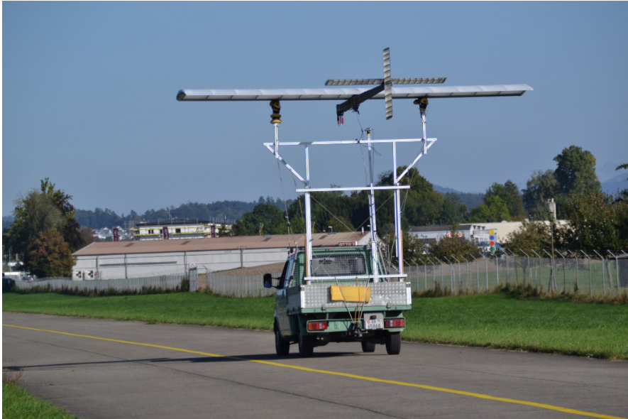
Fig. 24.12 Tow test on the former military airfield in Dübendorf, Switzerland, with a 6 m 2 twing
