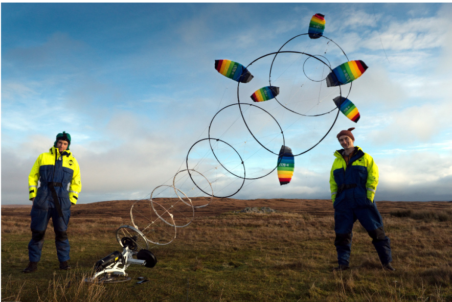
Fig. 21.13 Rotary ring kite stack in operation, generating P_{\text{net}} \approx 600 W, showing the portable tracking ground station, the new ring configuration and the force scale. Andrew Reeve (left) and the author (1 December 2017). See also [11]
