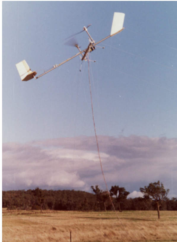
Fig. 23.7 The Gyromill Mk2 was equipped with twin, single bladed, counterweighted rotors of solidity 2.2% and a diameter of 3.65 m. The total mass of the craft was 29 kg. Again no cyclic pitch capability was employed. Thus in hover and wind it was found necessary to use three parallel tethers to maintain craft attitude. These three tethers were used in all tests, but the craft was difficult to control particularly in low winds. Two tethers were attached near the rotor thrust lines while the third tether was attached well forward on the forward pointing boom
