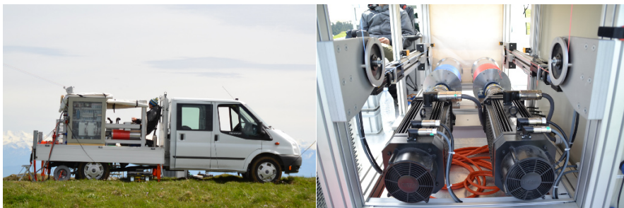
Fig. 24.1 Mobile ground station on the back of a truck (left) and in detailed view (right)
