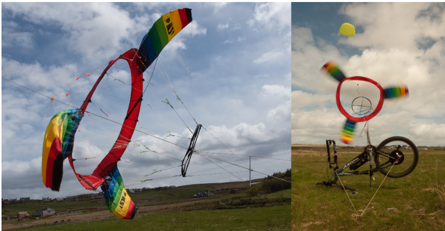
Fig. 21.4 A single daisy ring kite with three driver kites using two separated rotating tethers (“torque ladder”) to transmit rotational power to a ground-based generator (18 May 2015)
