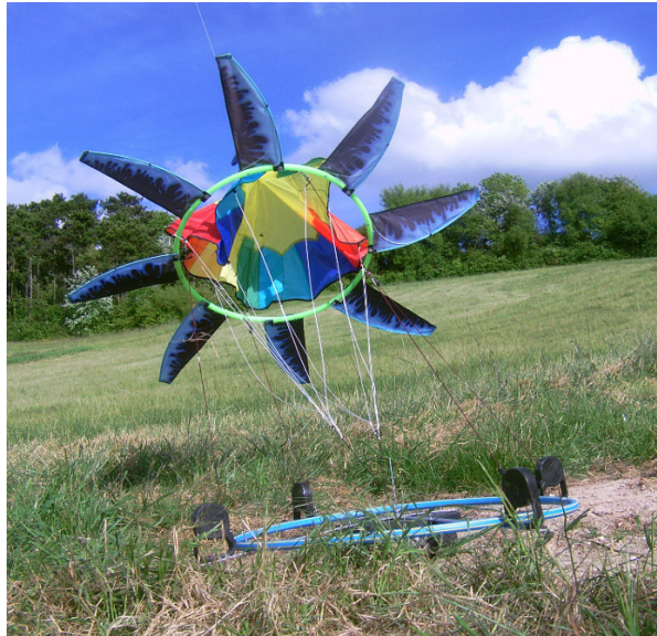
Fig. 22.7 Small-scale system built with two spars, a ring, four retractable leashes, a rotating tray, a parachute kite and semi-rigid rotor blades. The system uses four peripheral tethers and several suspension lines. The flying rotor measures 1.3 m from tip to tip
