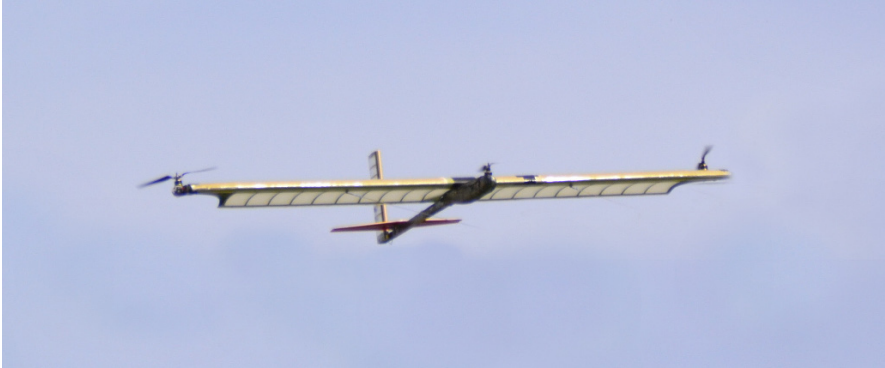
Fig. 24.5 Twing with integrated launching and landing concept in hover mode (2015)
