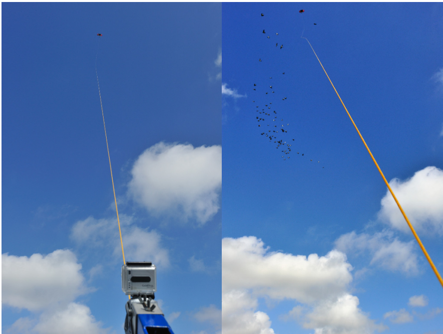
Fig. 28.3 Photo sequence capturing the rare situation of a bird, as part of a group of domestic pigeons ( Columba livia domestica ), impacting a tensioned tether, with the tether indenting and the bird recovering and continuing its flight. We can conclude that 1) birds can survive a tether impact and 2) the impact is clearly visible and may be used for monitoring. Depicted is the 20 kW kite power system of Delft University of Technology using a commercially available Genetrix Hydra LEI tube kite of 14 m 2 surface area, steered by a suspended remote-controlled control unit and a tether of 4 mm diameter made of Dyneema ® . The photo was taken on 28 June 2011 at Valkenburg airfield, The Netherlands, by Max Dereta
