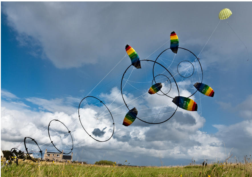
Fig. 21.2 The “daisy stack” developed by Windswept and Interesting Ltd employs a tensile structure to transmit the rotational power of stacked ring kite configurations (30 August 2017)
