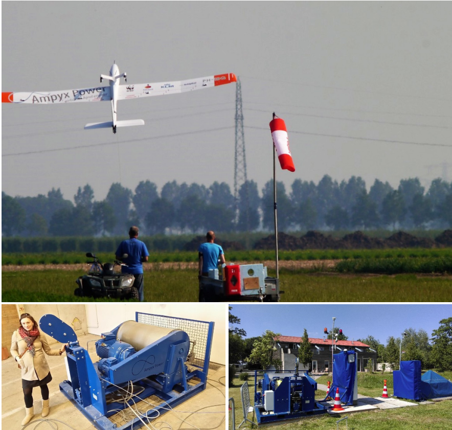
Fig. 26.4 AP-2A aircraft, 90 kW generator and control center
