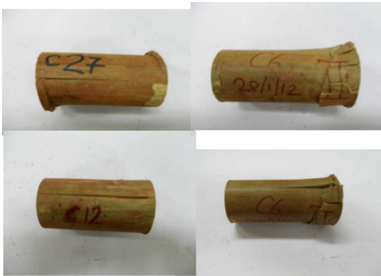
Fig. 18.1 Representative bamboo specimens tested for compressive strength
