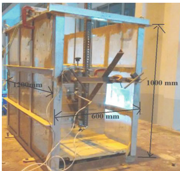
Fig. 13.12 Model container with model wall (After Reddy and Krishna 2015)
