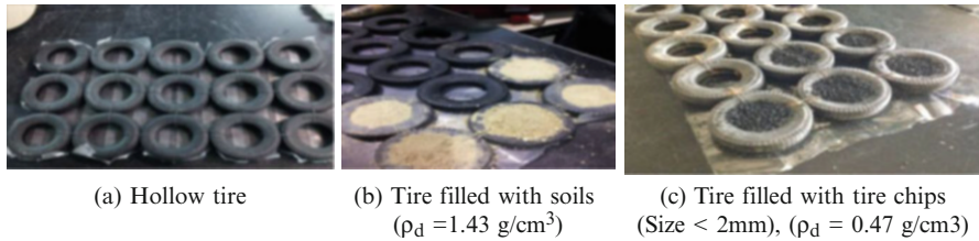
Fig. 9.17 Conditions of tire specimen according to filling materials. (a) Hollow tire. (b) Tire filled with soils ( \rho_d = 1.43 \text{ g/cm}^3 ). (c) Tire filled with tire chips (Size < 2 mm), ( \rho_d = 0.47 \text{ g/cm}^3 )
