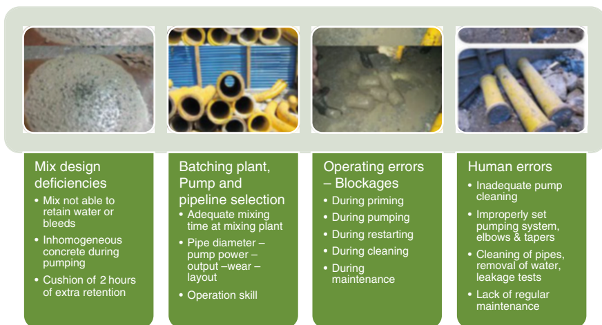
Fig. 20.7 Causes of pumping blockages
