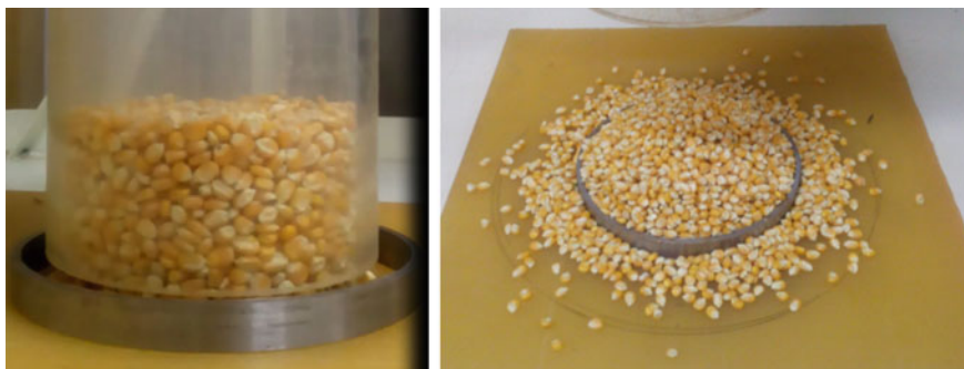
Fig. 1 The experiment of measuring angle of repose of corn
