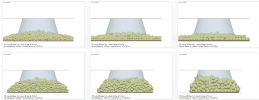
Fig. 5 Slump of particles for scale factor of \bar{\gamma} = \gamma S_f^3 and \bar{\gamma} = \gamma S_f
