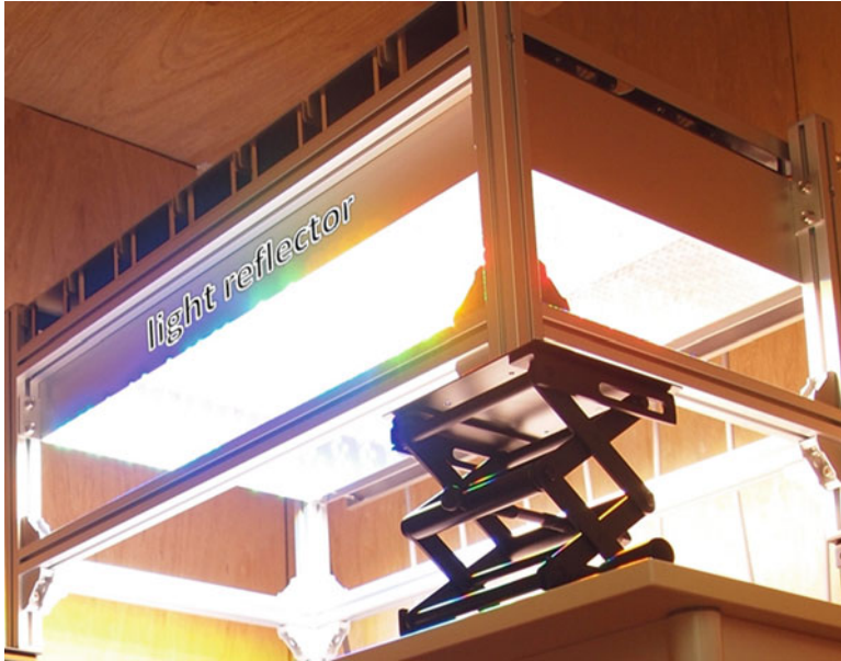
Fig. 30.2 Use of glossy light reflector surrounding the LED panel to increase light utilization
