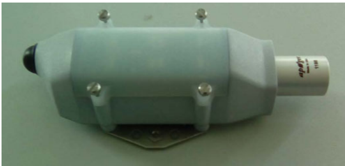
Fig. 1.2 Wireless sensor making measurements in pipe
