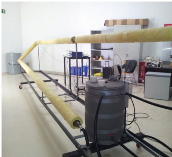
Fig. 11.3 Test rig: austenitic stainless steel pipes
