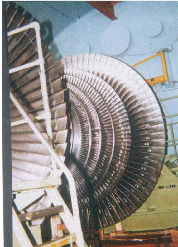
Fig. 1 Roter in balancing tunnel
