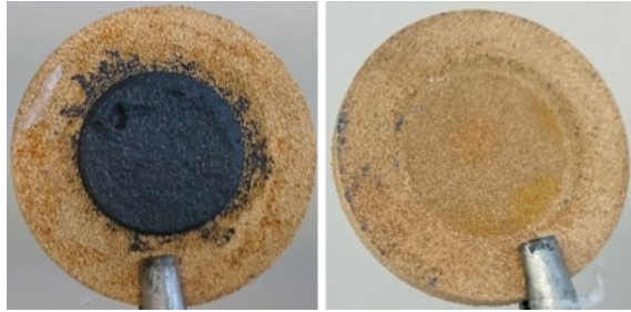
Fig. 2 Porous sample before and after surface cleaning
