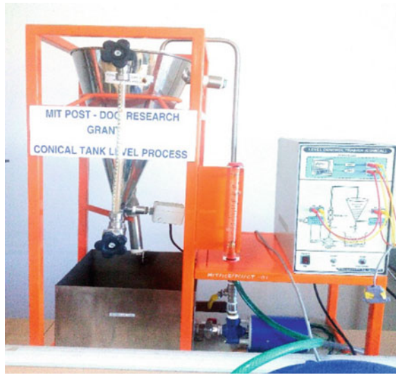
Fig. 2 Real-time setup for nonlinear level process
