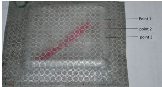
Fig. 7 Locations of strain measurement on the cup with one-fourth of height
