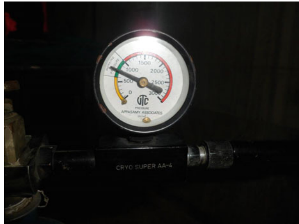
Fig. 14.5 Needle in pressure gauge should be in the green region
