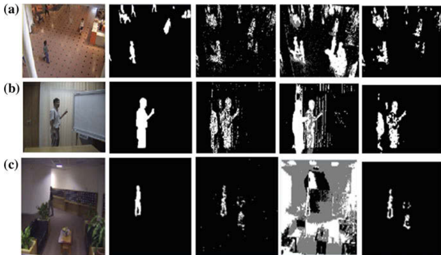
Fig. 2 Background subtraction results from left to right : i reference frame, ii ground truth, iii GMM, iv improved GMM, v proposed method
