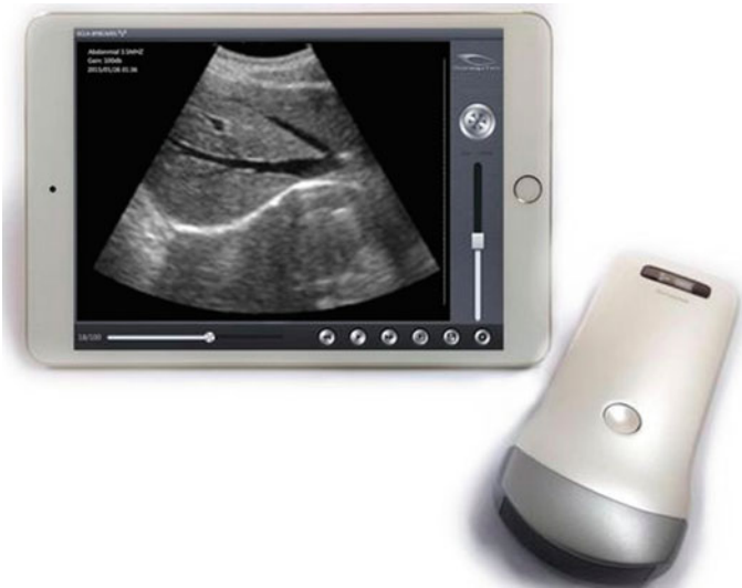
Fig. 5.2 Hand held wireless probe—connects to a tablet PC or a Smartphone with software [11]
