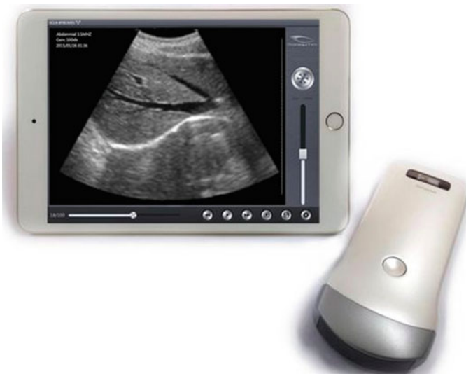
Fig. 5.2 Hand held wireless probe—connects to a tablet PC or a Smartphone with software [11]
