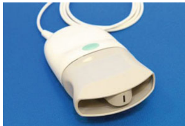
Fig. 5.3 The $50 ultrasound probe developed by Newcastle University, UK [12]
