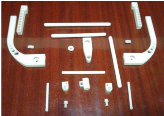
Fig. 19 Links of each one of the distractors (printed by Stereolithography)
