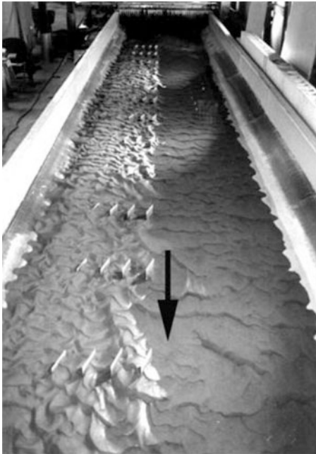
Fig. 13.3 Upstream view of nearly drained, straight channel with vanes (Source: Odgaard and Wang (1991a), ASCE)
