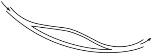
Fig. 13.14 Stabilization by channel split
