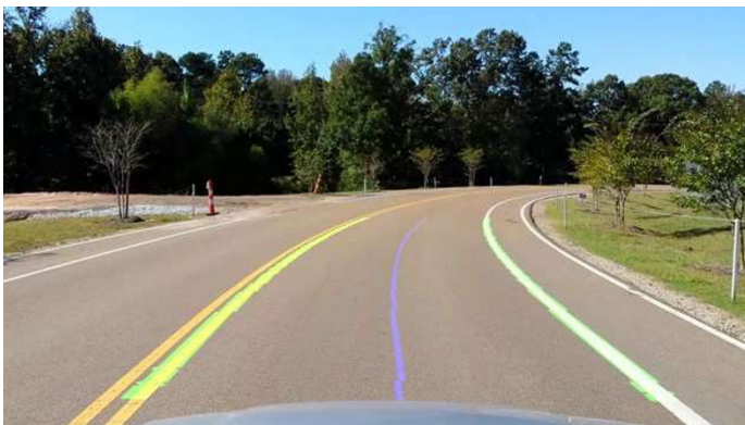
Fig. 5. Final lane detection overlaid to live camera image.
