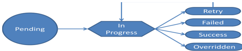
Fig. 6. Lifecycle diagram of "syncStatusId" field
