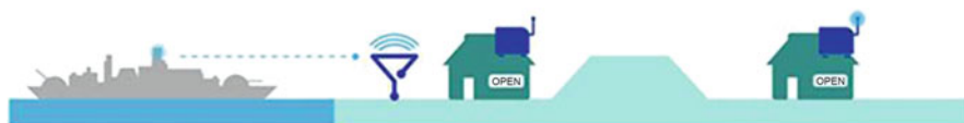
Fig. 6 CBRS spectrum sharing scenario in 3.5 GHz between an incumbent system (in this case Navy radar) and secondary users
