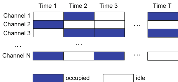
Fig. 13 Channel model for cognitive radio
