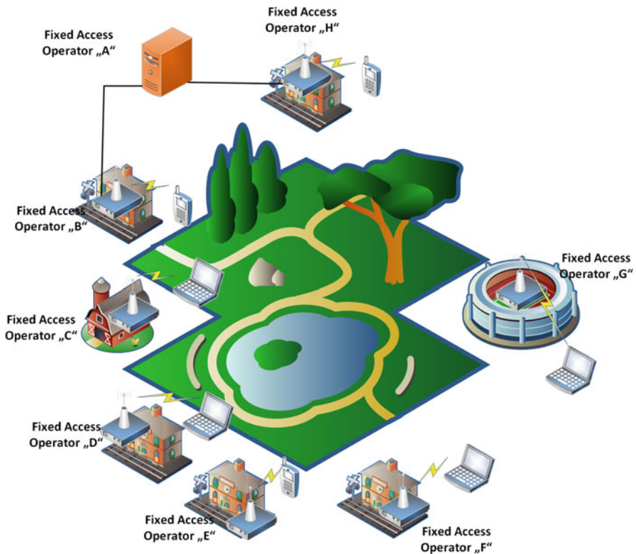
Fig. 9 Use case scenario of internet access by hybrid of networks with distributed and centralized coexistence managements on (TV) White Space frequency bands
