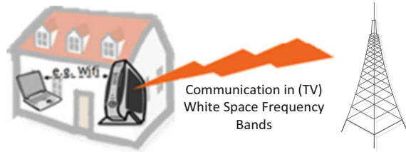
Fig. 6 Mid-/long-range wireless access, no mobility
