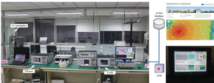
Fig. 16 CR-enabled TD-LTE test-bed
