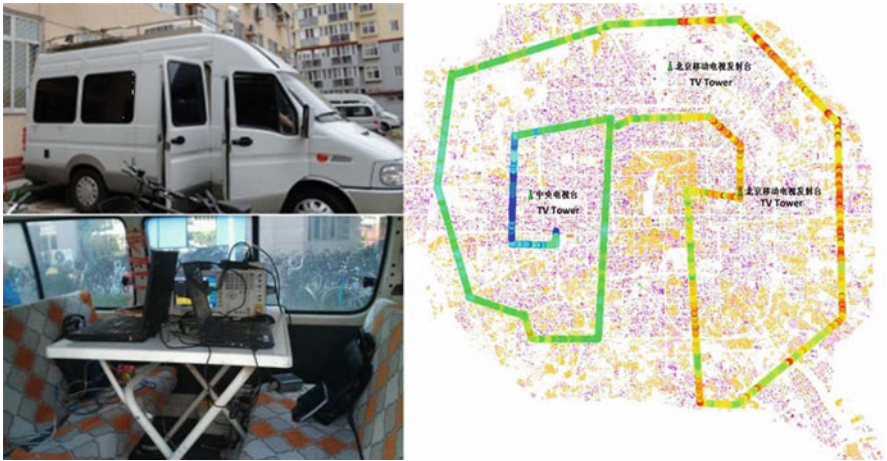
Fig. 2 Equipment and route of mobile measurement
