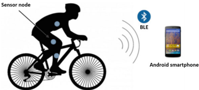
Fig. 1 Architecture of the developed cycling posture monitoring system
