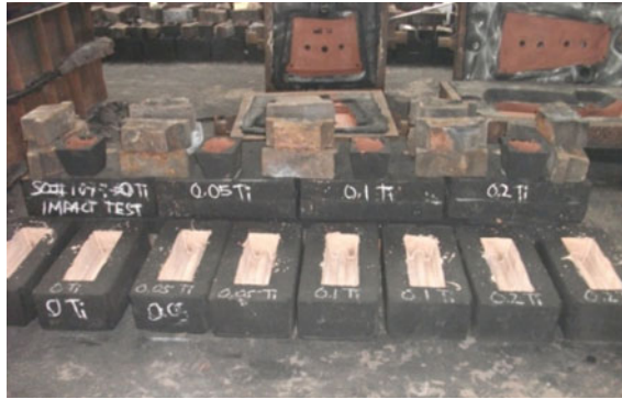
Fig. 1 Furan sand molds being utilized in the production of manganese steel
