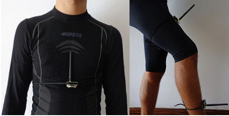
Fig. 7 Sites of placement of the sensors on the athlete's body: torso ( left ) and leg ( right )
