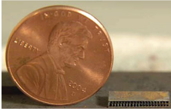
Fig. 50 CVD diamond microchannel cooler with 250 \times 300 \mu\text{m} rectangular ducts [209]
