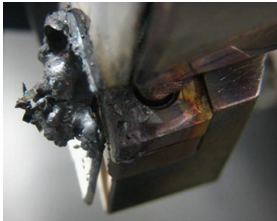
Fig. 19 Damage in the cutting tool when the laser beam is focused at a circumferential distance of 25 mm from the cutting tool [97]
