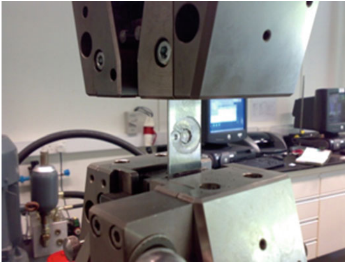
Fig. 2 A photograph of lap shear test
