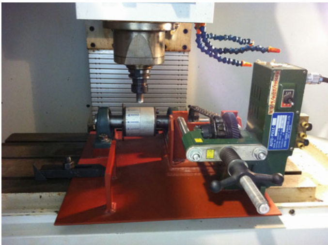
Fig. 1 Orbital clamping unit for friction stir welding of aluminium pipe
