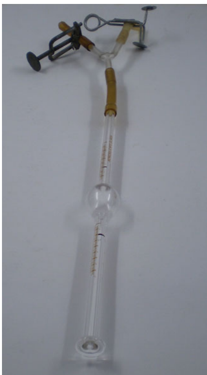
Fig. 8.2 Traube's stalagmometer used to measure surface tension by the drop-weight and drop-count methods
