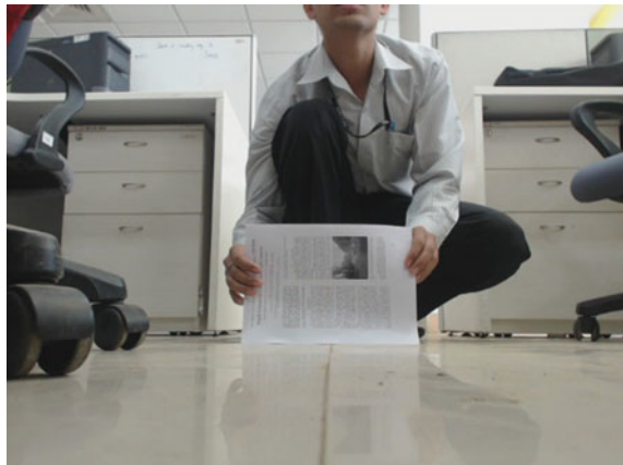
Fig. 4 Captured object at known distance to find the focal length of the camera
