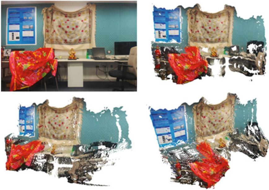
Fig. 3 Topleft sample image for reconstruction, Rest 3D point cloud after reconstruction
