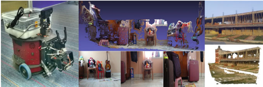
Fig. 1 Left to right figure shows the Firebird VI robot used in our experiments, sample data sets and corresponding reconstructions
