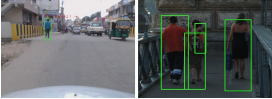
Fig. 8 Detection on real video frame and INRIA dataset image with low illumination
