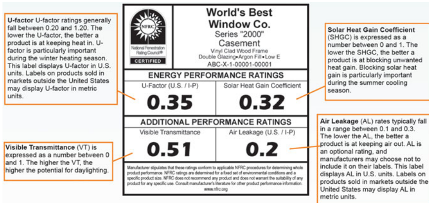
Fig. 4.12 Example of a NFRC rating label to understand the energy performance of windows (NFRC 2012)
