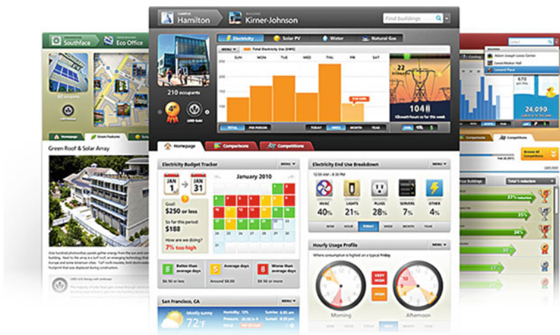
Fig. 6.4 Example of building monitoring dashboard (CCS 2013)
