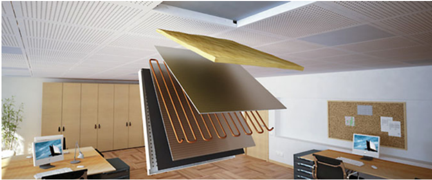
Fig. 5.7 Chilled ceiling panel components (SGL Carbon 2012)
