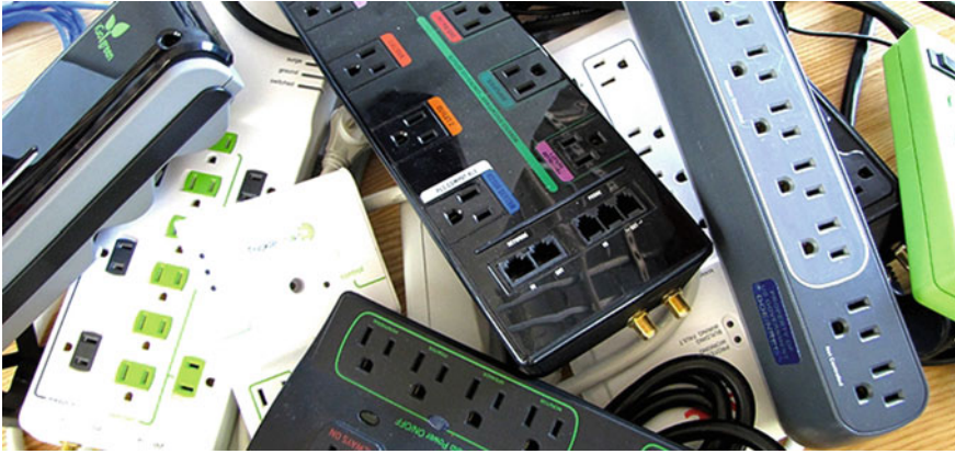
Fig. 5.18 Different types of smart/advanced power strips (Source Earle and Spahn 2015)
