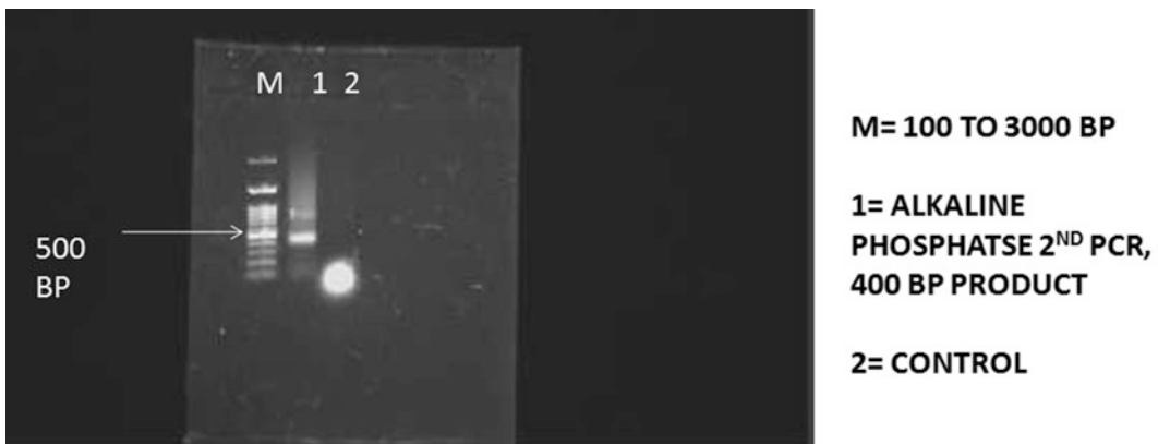
Fig. 10.1 2nd PCR from alkaline phosphatase from 1st PCR sample. Using 1 % agarose gel. For image analysis, Gel Doc (Bio Rad, Serial no. 76S/08119, software Quantity One, version 4.6.3)
