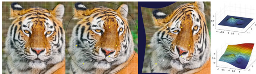
Fig. 1 From the left , the original image, images warped by 2D biharmonic clamped plate spline (CPS) and thin plate spline (TPS). Control point correspondences ( small squares ) are indicated as yellow (source) and white (target). The right most image is comparison of the CPS ( top ) with TPS ( bottom ) interpolating the same points. The CPS is both smooth and localized, decaying to zero at the boundary of the unit disc
