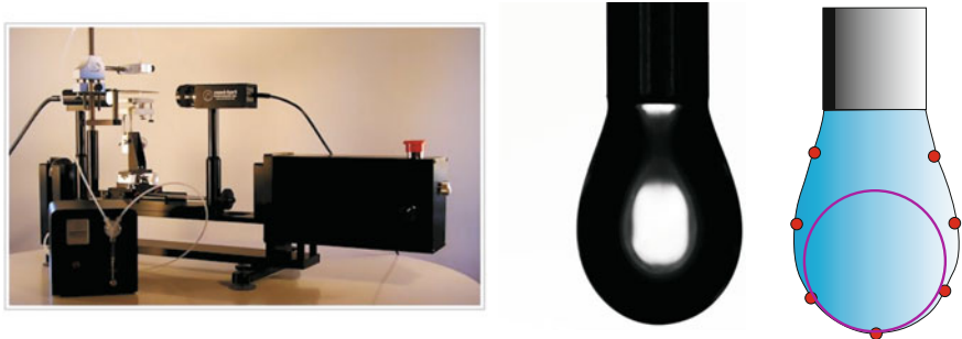
Fig. 4 Left description of the typical apparatus of the pendant drop method. Right a pendant drop is modeled by an axisymmetric surface by adjusting its contour
