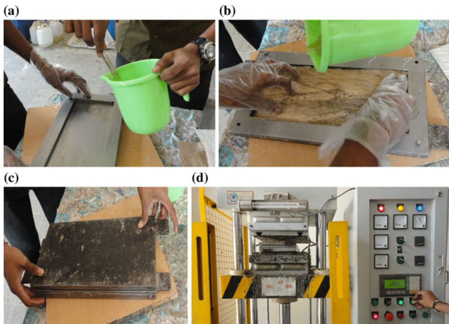
Fig. 1 Steps involved in fabrication process. a Positioning of mold. b Fiber arrangement. c Closed mold. d Mold placed in the compression machine
