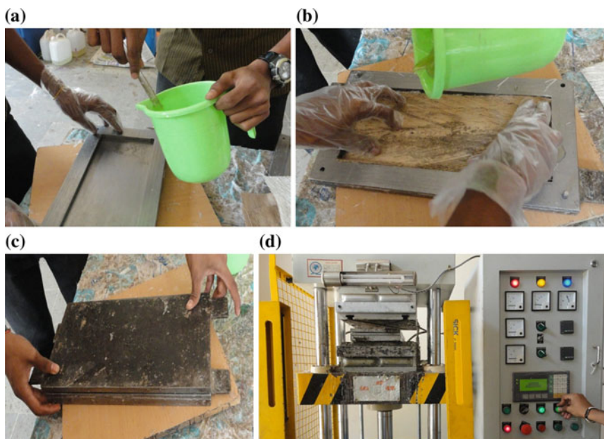
Fig. 1 Steps involved in fabrication process. a Positioning of mold. b Fiber arrangement. c Closed mold. d Mold placed in the compression machine
