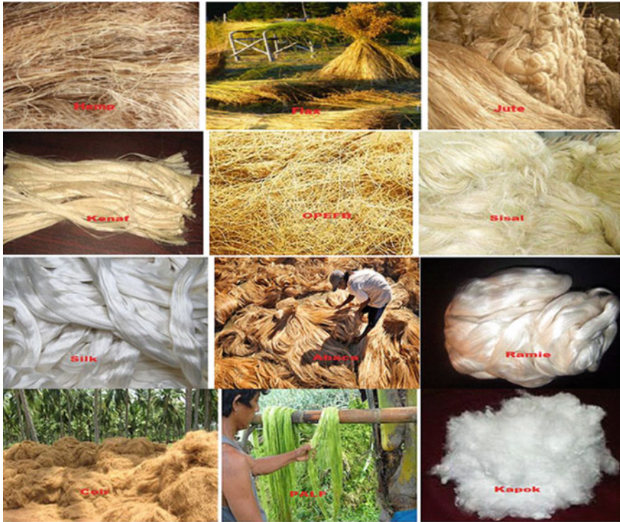
Fig. 1 Different types of natural fiber used as reinforcement
