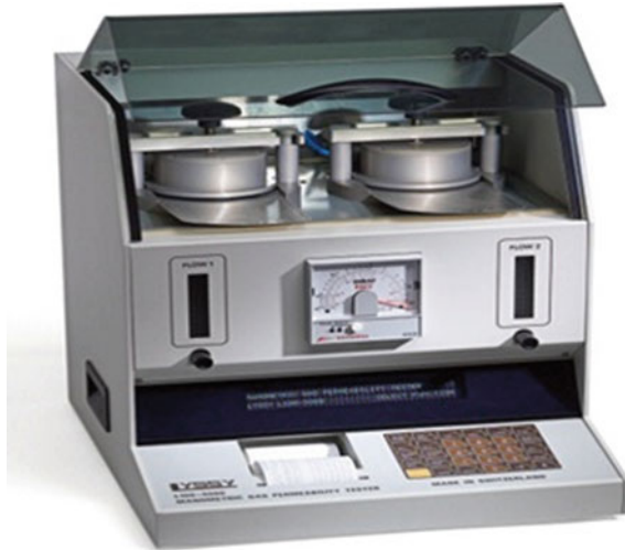
Fig. 4 Gas permeability measuring unit
