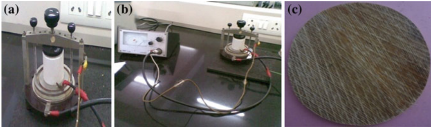
Fig. 6 a Connections between the power supply and the ohmmeter. b Resistivity adapter. c Disk shaped sample
