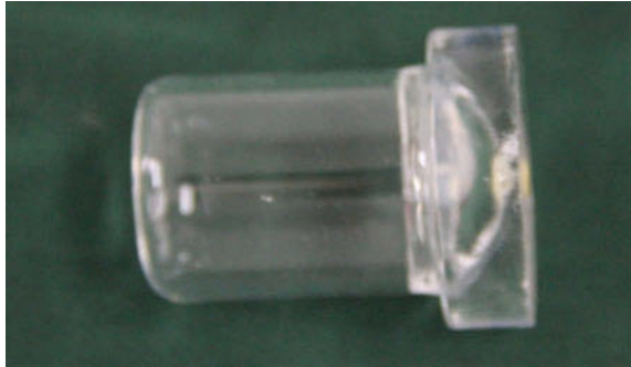
Fig. 1 The discharge bulb of hydrogen maser
