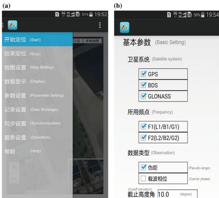
Fig. 3 The operation interface of the software (a) The interface for positioning parameter configuration (b)
