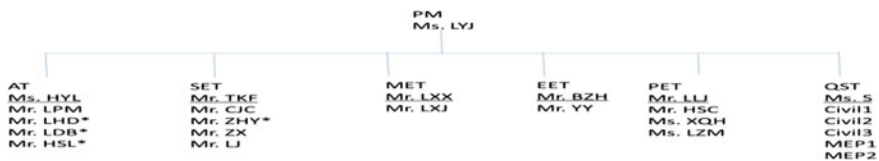
Fig. 91.3 Project organization chart. Notes (1) AT architecture team; SET structure engineering team; MET mechanical engineering team; EET electrical engineering team; PET plumbing engineering team; QST quantity surveying team; (2) *staff from City C 3. Name with underlying denotes discipline leader
