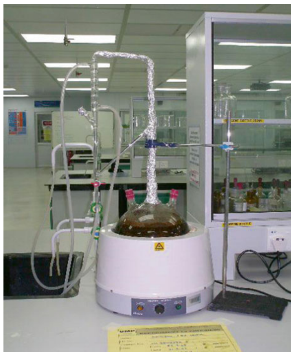
Fig. 7.3 Hydrodistillation using Clevenger-type apparatus
