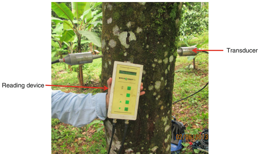
Fig. 9.3 A field test using the NDT technology of Sylvatestduo® acousto-ultrasonic equipment
