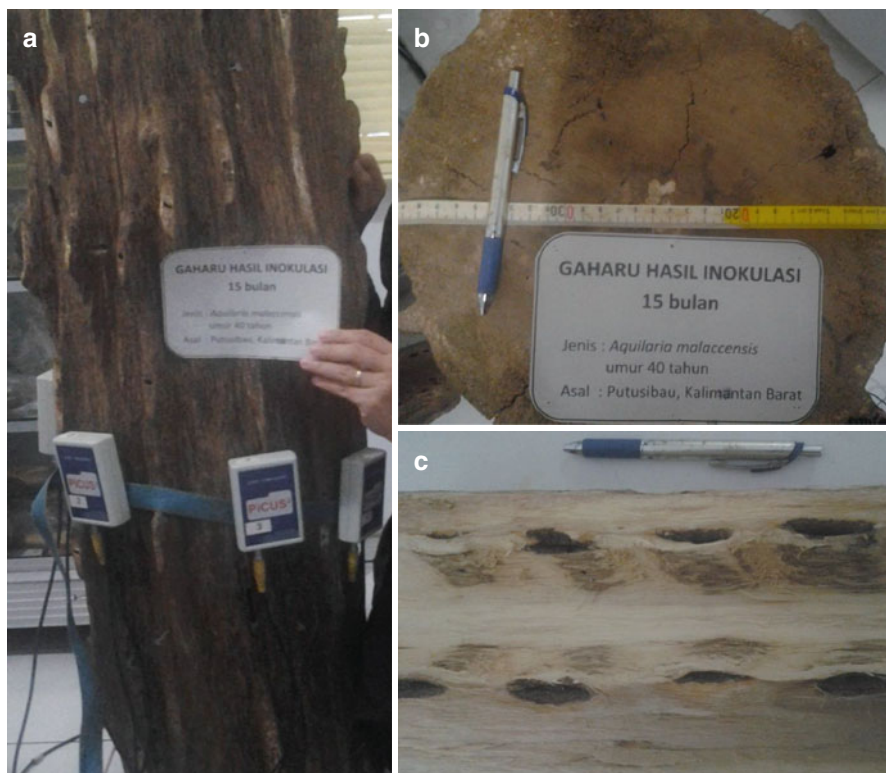
Fig. 9.8 A trunk of Aquilaria malaccensis harvested 15 months after inoculation using FORDA's technique. (a) PiCUS® sonic tomograph sensors were installed on the trunk, (b) trunk diameter of 32 cm, and (c) visible presence of agarwood in the trunk
