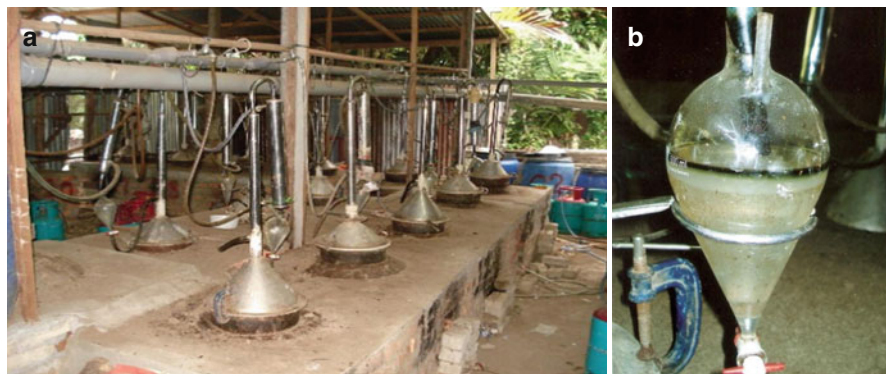
Fig. 7.2 A commercial hydrodistillation system for agarwood oil extraction in Gua Musang, Kelantan (Malaysia). (a) Extraction contraption and (b) extracted oil in the collecting cone
