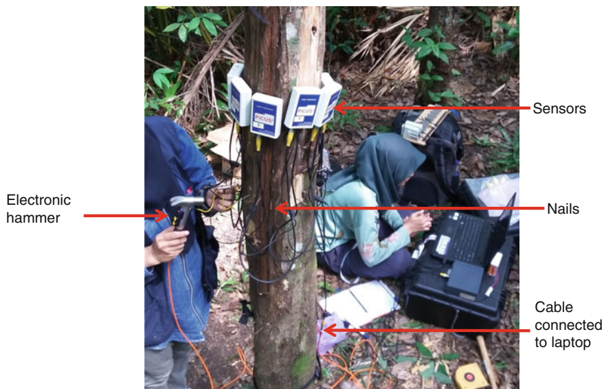
Fig. 9.4 A field test using the NDT technology of PiCUS® sonic tomograph
