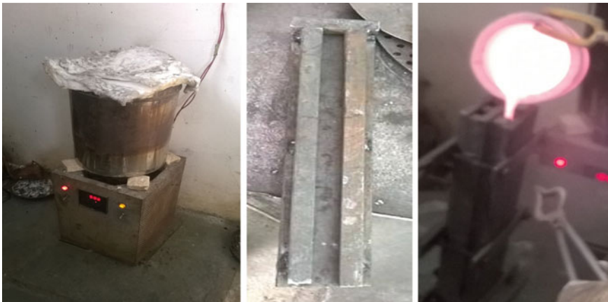
Fig. 2 Electric muffle furnace, Mould, and Casting process
