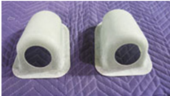
Fig. 7 FDM-layup tool produced the aircraft camera fairings
