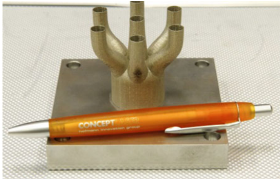
Fig. 4 The first test piece produced on the M2 curing machine (Courtesy NASA/MSFC/Andy Hardin)
