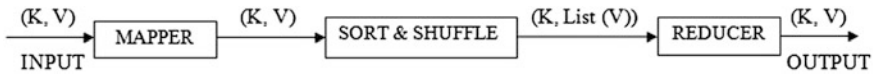
Fig. 1 The figure shows the working of the mapreduce framework. The input and output are both in the form of key-value pairs
