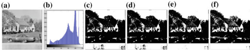
Fig. 3 a Original image, b histogram, c segmented image using Shannon entropy, d segmented image using collision entropy, e segmented image using min entropy, f segmented image using Renyi entropy
