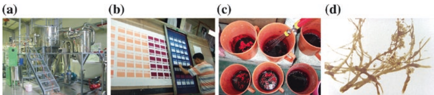
Fig. 13 Whasoomok's natural DTP processes. a Spray-drying instrument. b Natural color sampling. c Color making. d Natural DTP sample made with acacia, nutgall, and marigold (Whasoomok 2015)
