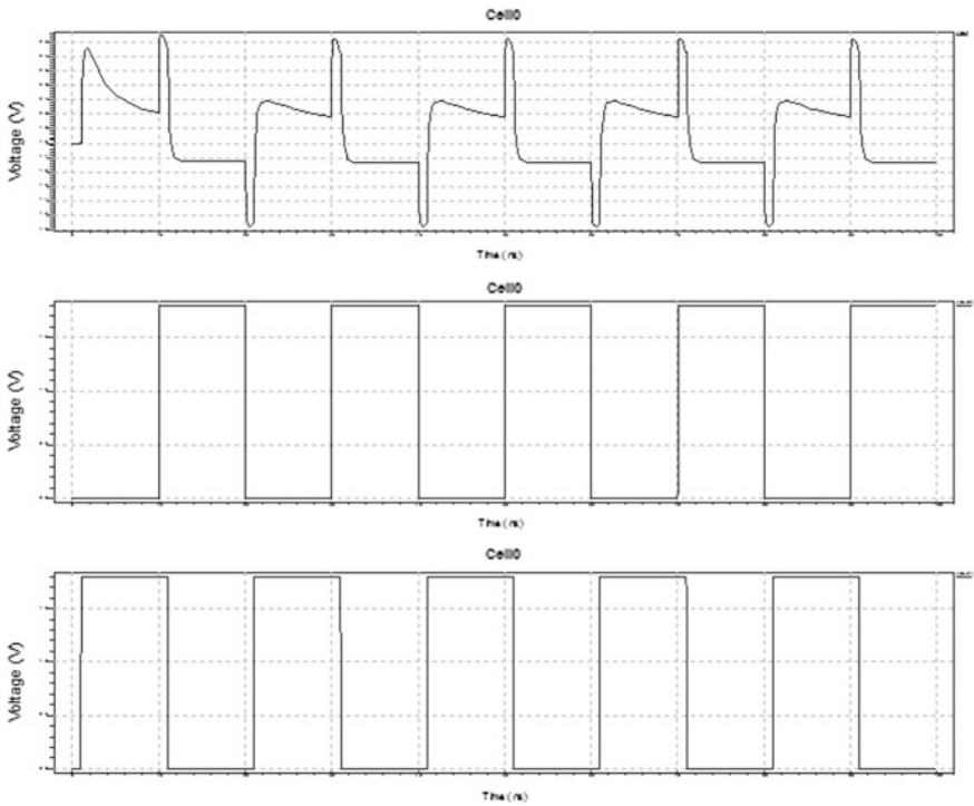
Fig. 6 Output waveform of dynamic charge transfer switch
