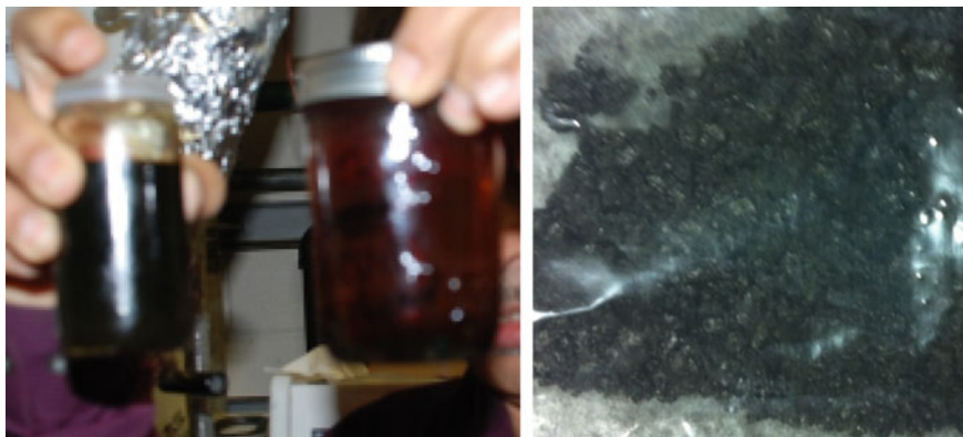
Fig. 5 Biooil ( left ), bioliqor ( middle ) and biochar ( right ) samples from BLT press cake
