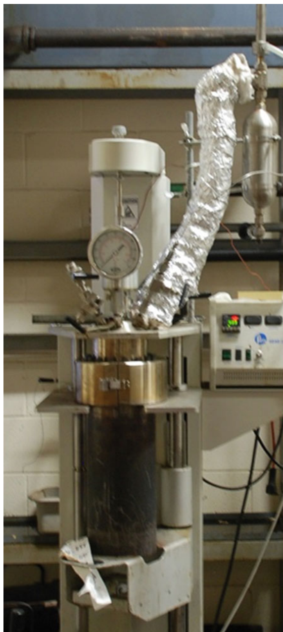
Fig. 3 Batch pyrolyser used in the thermal conversion of BLT press cake
