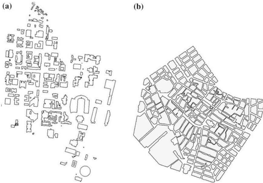
Fig. 13.2 Building footprints as extracted from OpenStreetMap data. a University of Texas at Austin. b Downtown Vienna
