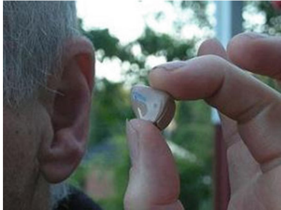
Fig. 12 Customised in-the-ear hearing aids made using 3DP [7]
