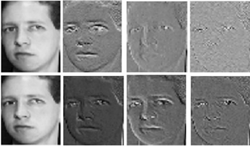
Fig. 4 The decomposition results (at level 1) using our weighted adaptive scheme and the wavelet transform used in [11]. Top (from left to right): the approximate, horizontal, vertical and diagonal detail images of the wavelet transform. Bottom (from left to right): the approximate, horizontal, vertical and diagonal detail images of our weighted adaptive scheme
