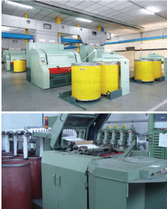
Fig. 9 A high-speed carding machine ( top ) and a gill-drawing machine. Source The top image is from Melland International 3 (2011) 133. Published with the authorization of Deutscher Fachverlag GmbH, Germany. The bottom image is from the author’s personal collection
