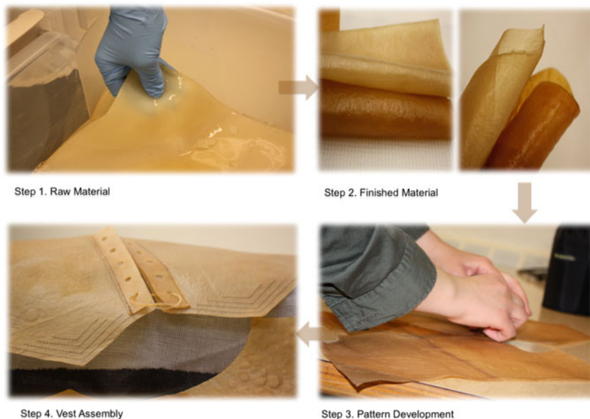
Fig. 8 Process of developing new bacteria cellulose nonwoven material and vest prototype. Source Image by the author, Young-A Lee, April 15, 2015
