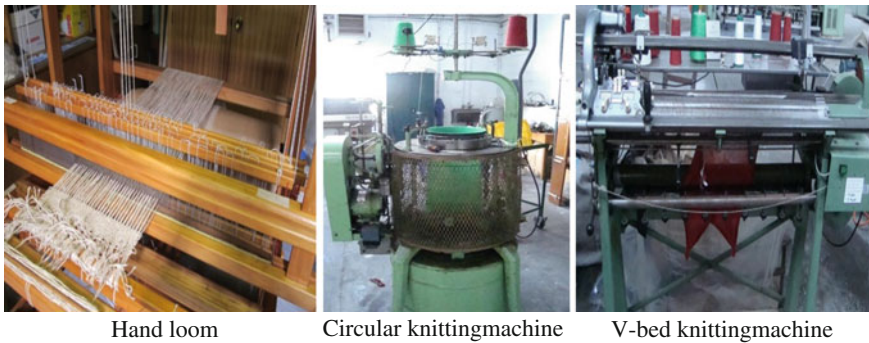
Fig. 11 A handloom, a circular single-jersey knitting machine, and a V-bed knitting machine. Source The author’s personal collection
