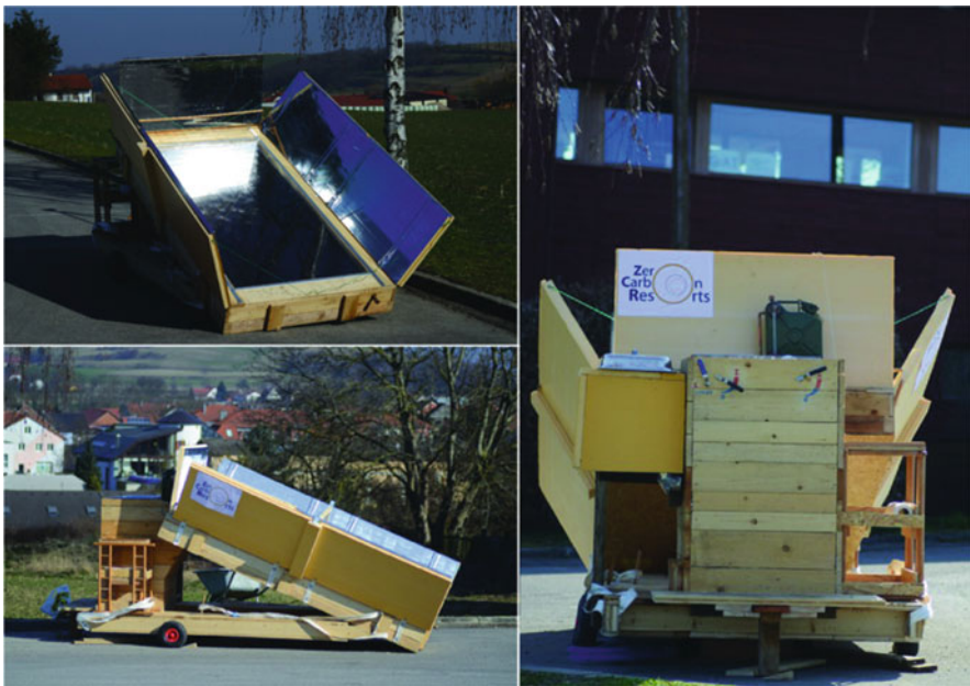
Fig. 5 Flat-plate collector with indirect solar cooker prototype
