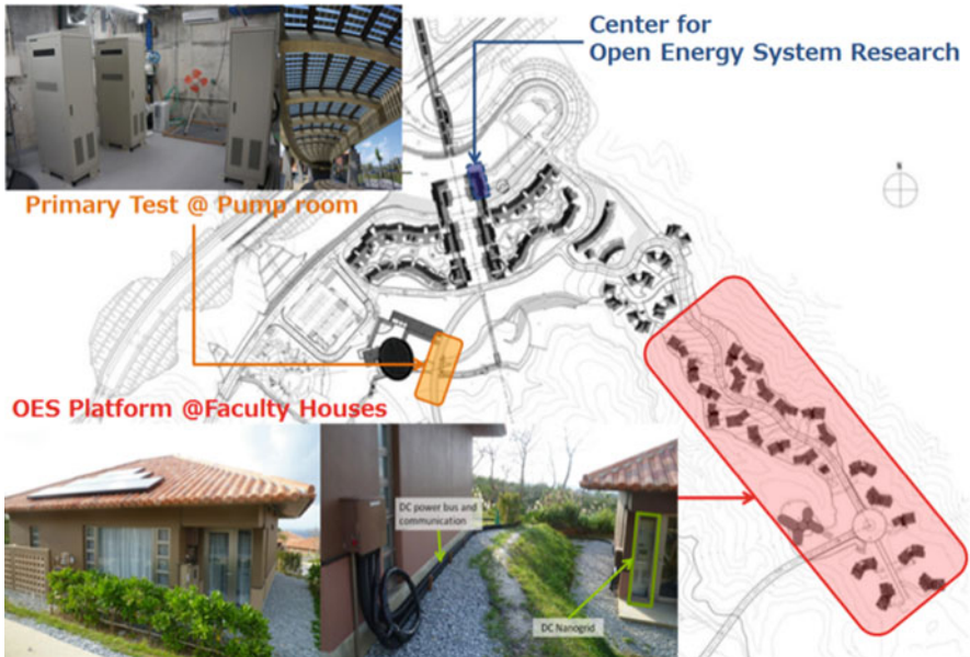
Fig. 13 OES platform at OIST: primary test site and full-scale platform at faculty houses
