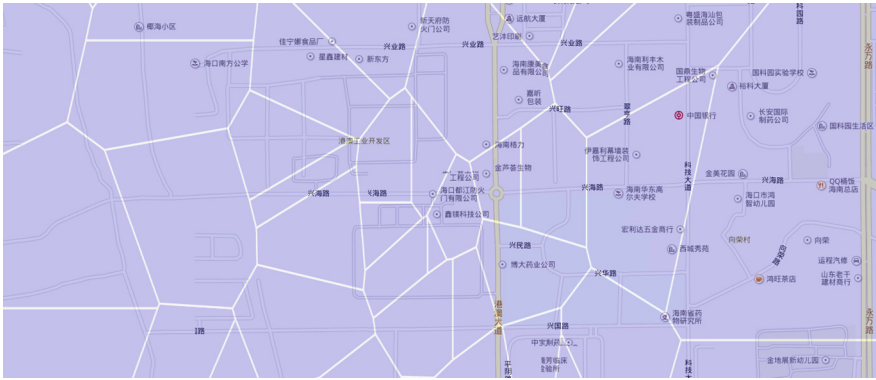
Fig. 2. Actual service coverage divided by Thiessen polygon in cellular network.
