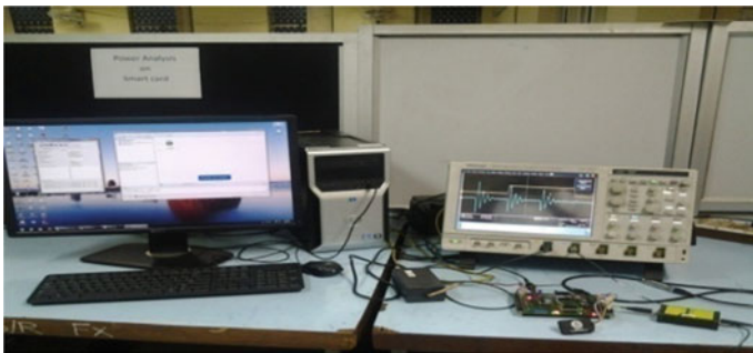
Fig. 2 Lab setup for acquisition of power signal
