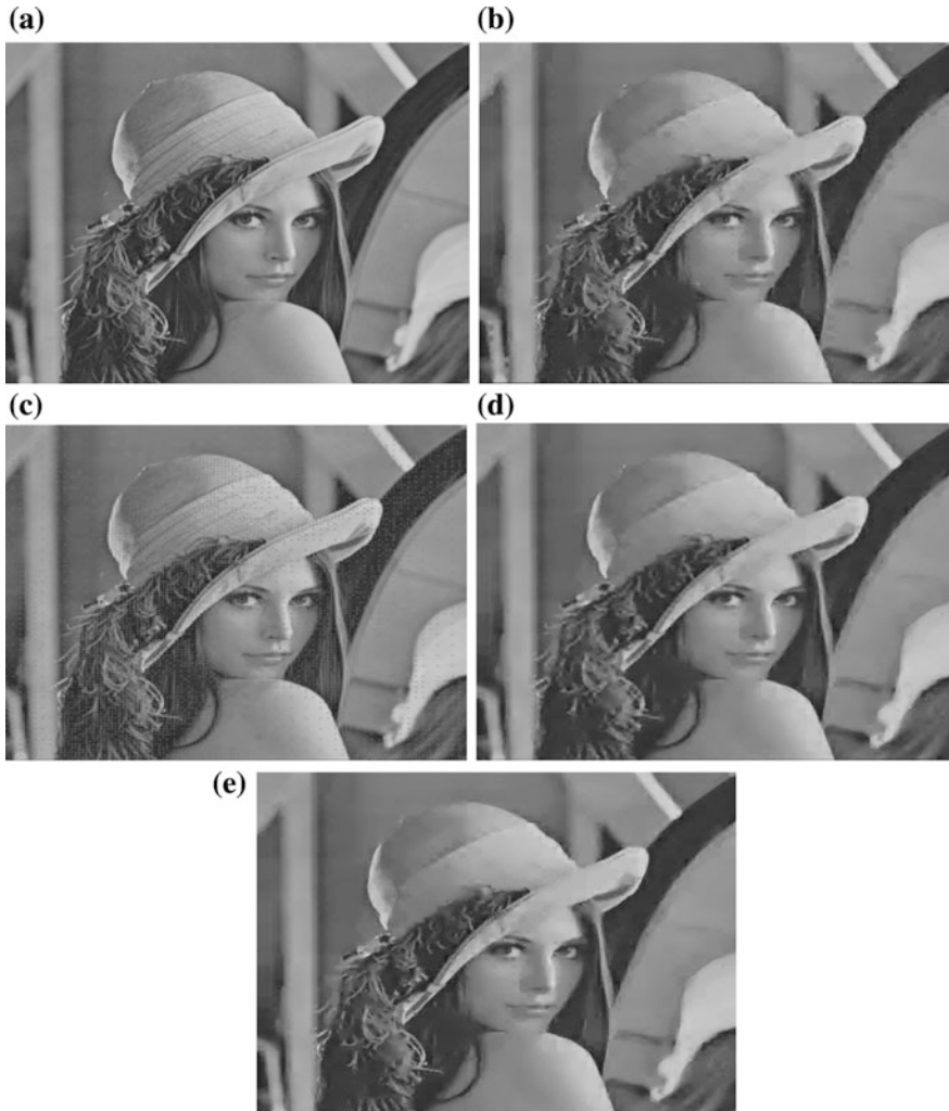
Fig. 3 Experimental results of image encoding: a original image b is image decoded using no search in DCT domain c decoded image using no search using fast DCT d image decoded using range exclusion method e image decoded using no search real DCT method
