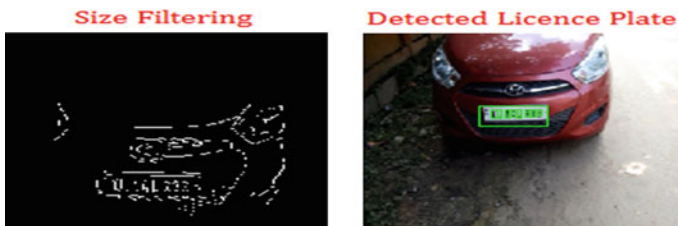
Fig. 2 Size filtering and genetic algorithm phase to detect the registration plate in MATLAB
