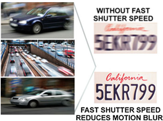
Fig. 4 Example showing how fast shutter speed cameras reduce motion blur ( http://www.licenseplatesrecognition.com/hardware-involved-in-lpr.html )
